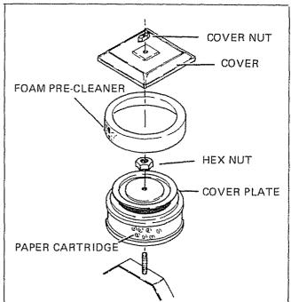
Once yearly or every 100 hours of operation (whichever comes first), remove hex nut, cover plate, and paper cartridge. Clean paper cartridge by tapping gently on a flat surface. If extremely dirty, replace cartridge or wash cartridge in liquid detergent and water. Rinse cartridge until water remains clear. AIR DRY CARTRIDGE THOROUGHLY BEFORE USING.
